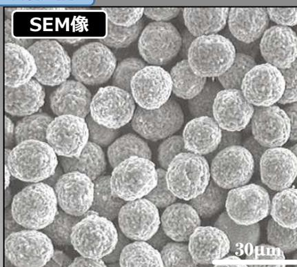
基材: LiNi<sub>0.33</sub>Co<sub>0.33</sub>Mn<sub>0.33</sub>O<sub>2</sub> 粉末
