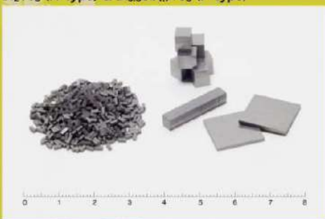
\text{Bi}_2\text{Te}_3 (N-type) & \text{Bi}_{0.3}\text{Sb}_{1.7}\text{Te}_3 (P-type)
