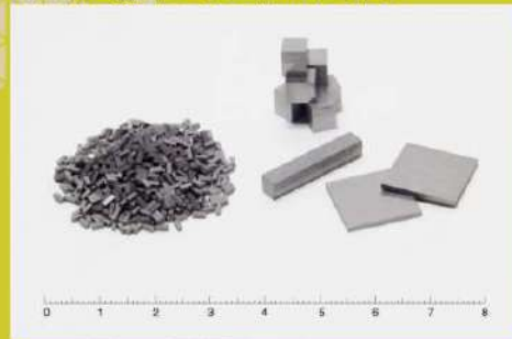
\text{Bi}_2\text{Te}_3 (N-type) & \text{Bi}_{0.3}\text{Sb}_{1.7}\text{Te}_3 (P-type)
