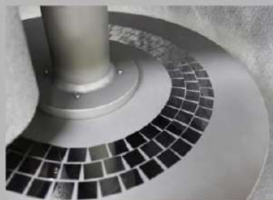
Stage where three rows of 10mm square substrates are installed
