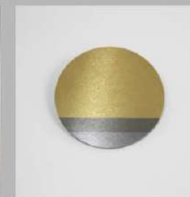
Au/Ni/thermoelectric material (3 layers)
