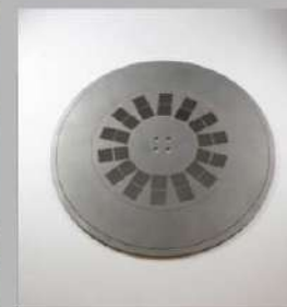
Stage where two rows of 10mm square substrates are installed
